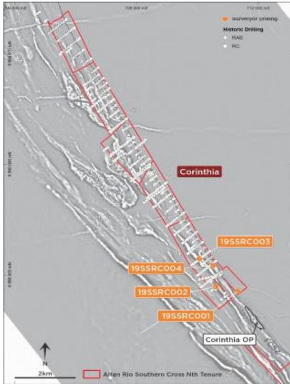
Figure 2: Corinthia North Drill Hole Location Plan
